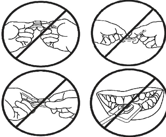
3. There is a risk of cable breakage when excessive force is applied while pulling down or holding the sensor cable.
